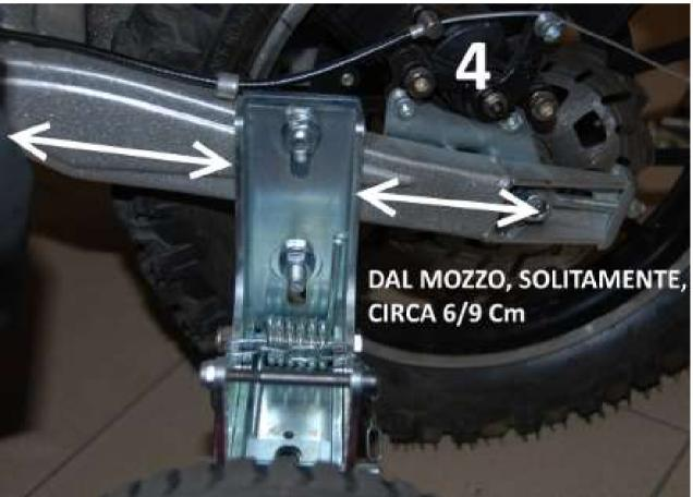
3 IDENTIFYING THE CORRECT POSITION OF THE FIRST TWO HOLES TO BE PRACTICED ON THE SUPPLIED PLATE:
