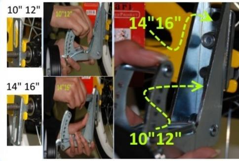
Warning !before attacking the destabilizers you have to charge the spring as in the picture above (step 1). For the bikes 14" the wheel shall stand slightly up and it 'll touch the ground because of the weight of the child after the spring adapted as in the step 2. To attack the destabilizers on the bike follow the instructions given by the producer and check the way of the pedals: right and left!
